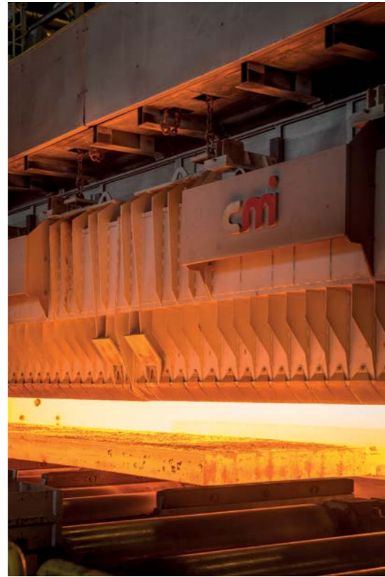
A steel slab exits the new, energy efficient walking beam furnace (Ghent).
