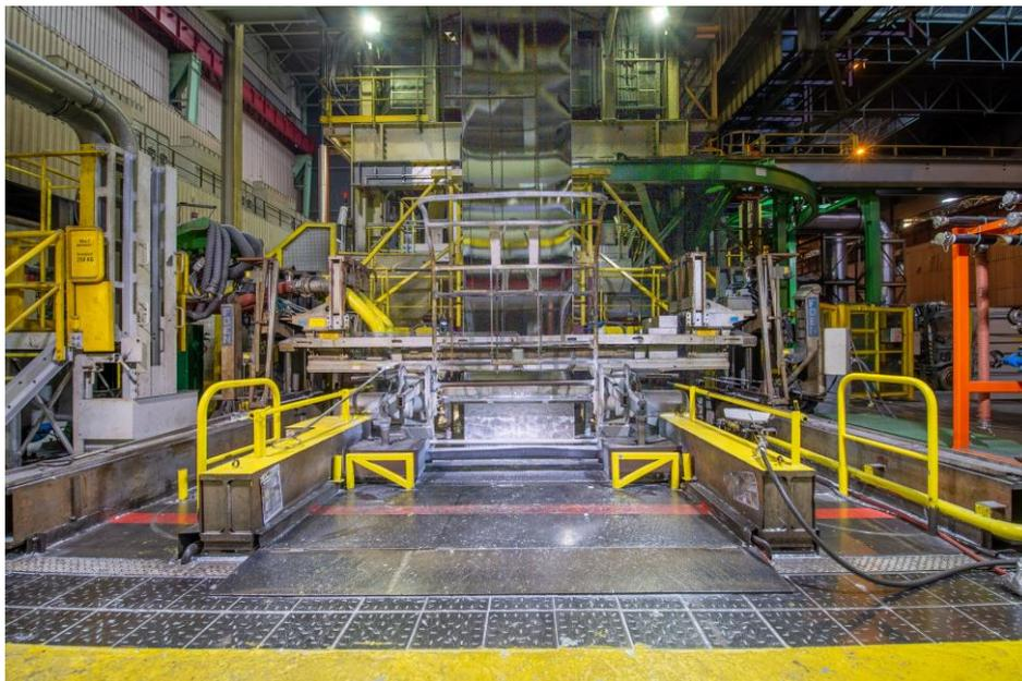
3 - The zinc bath of Sidgal 1, in which the steel is coated.
